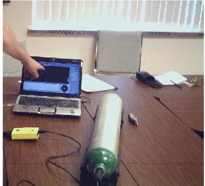
Visual Eddy test set up on O2 tank
