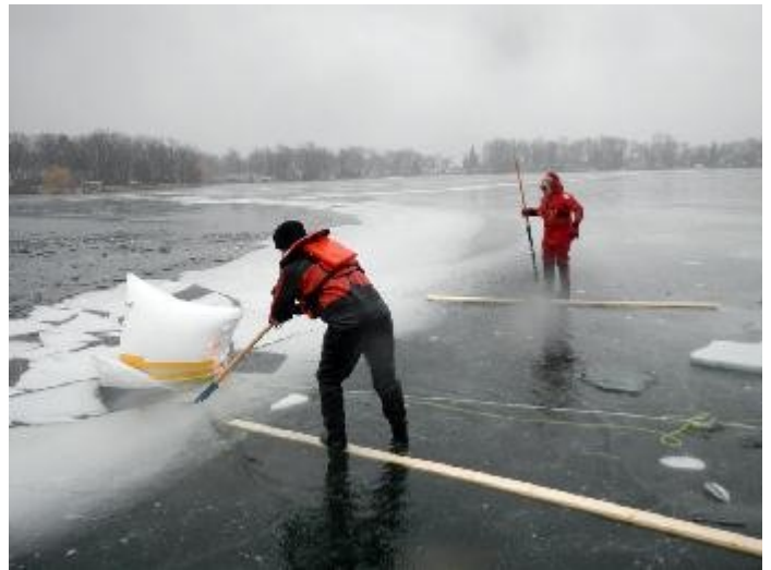
Floated up with airbag, snowmobile needs a path through ice
