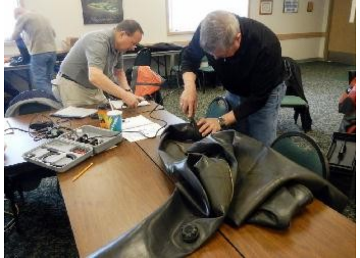
Ken Kruska and Mike Fabish use Dremel tools to roughen a suit prior to gluing on a wrist seal
